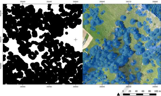
Figure 6: (Left) Creating a buffer area around objects by using the *Proximity (Raster Distance) analysis* tool. (Right) Identification of trees and buildings and vectorialization of raster in shape file layer.
