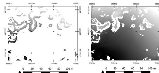
Figure 3: Example of Removed objects and Bare-Earth, the output from a DTM filter slope-based.
