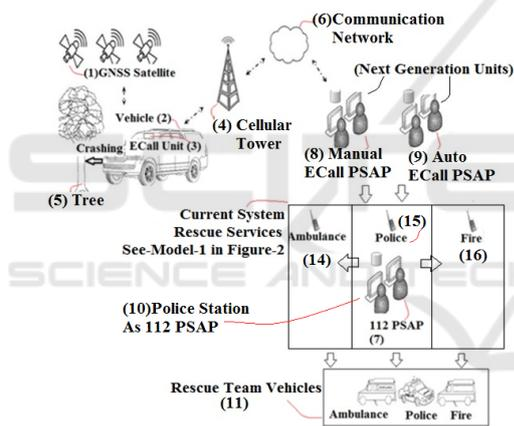
Figure 1: Generic eCall crash notification system for Italy (Current and Next Generation Units).
