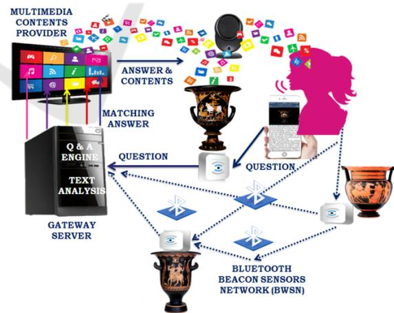
Figure 3: Service System Architecture.
