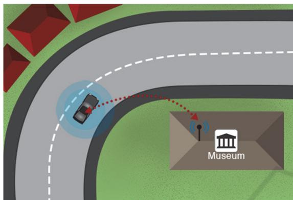
Figure 1: Infotainment. A car drives through an unknown city and gets information via V2X-technology.
