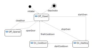
Figure 8: Superimposed statechart realizing feature "Microwave Oven" in concrete graphical syntax.
