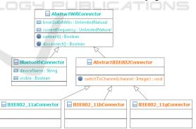
Figure 4: UML2 class diagram showing the realization of wireless connections in the multi-variant domain model.
