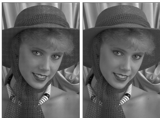
Figure 3: On the left an example of a CFA image. On the right, the obtained grayscale image using directly the CFA image.
