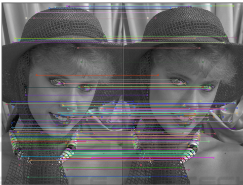
Figure 11: Match SURF Keypoints for image 04 of the Kodak set (on the left) using FLANN algorithm considering the CFA image (on the right). The complete results can be found in http://sweet.ua.pt/an/FullResults.zip .
