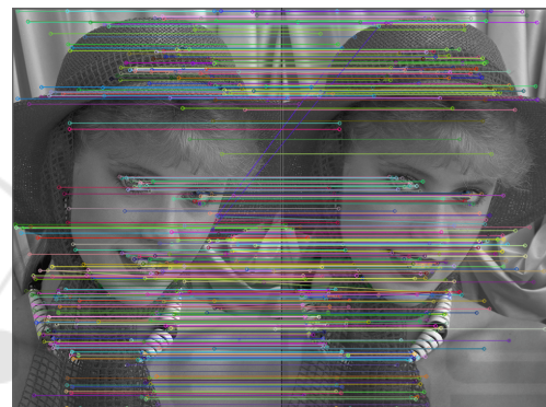
Figure 14: Match SIFT Keypoints for image 04 of the Kodak set using FLANN algorithm. The complete results can be found in http://sweet.ua.pt/an/FullResults.zip .
