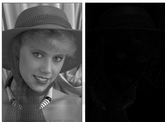
Figure 4: On the left, the grayscale image obtained from the full RGB image. On the right, the difference between the image on the left and the grayscale image obtained from the CFA image presented in Fig. 3.
