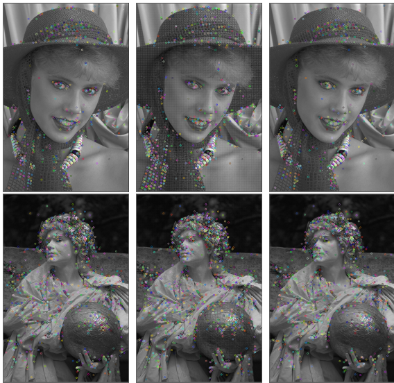
Figure 6: SURF Keypoints for for images 04 (first row) and 07 (sencond row) of the kodak set. The complete results can be found in http://sweet.ua.pt/an/FullResults.zip .
