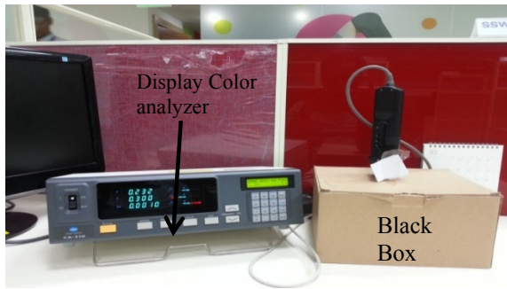
Figure 13: Setup for generating panel tuned look-up table.
