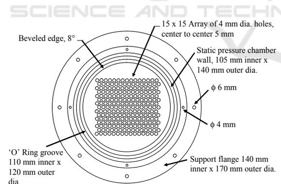
Figure 2: Pressure sensor layout.
