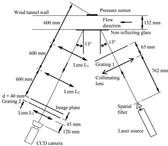
Figure 4: Optical setup used for creating moiré fringes.
