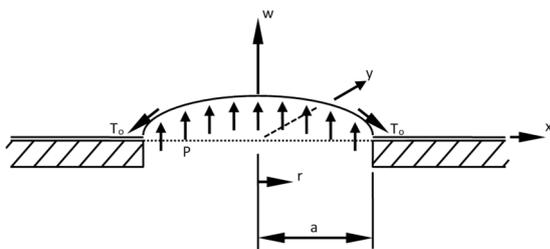
Figure 5: Elastic membrane stretched over a pressure sensor.
