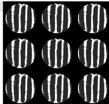
Figure 6: Constant slope moiré fringes recorded over a 3 x 3 version of the pressure sensor.
