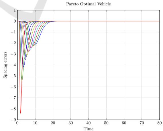
Figure 8: Performance of the Pareto optimal controllers ( $\tau = 0.5$  s,  $L_{des} = 40$  m,  $h = 0.9$  s,  $k = 10$ ,  $\lambda = 1.6$ ). The different lines correspond to the spacing errors of each Pareto optimal vehicle in the stream.
