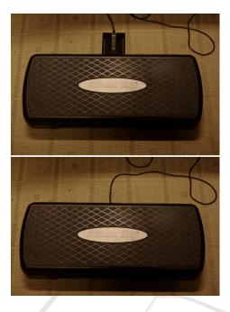
**Fig. 5.** Experimental setup used in the studies following the NIW project. A microphone was placed below a stepper to detect person's steps. An actuator was located under the top layer of a stepper [7].
