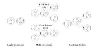
Figure 3: Basic structures of logistics systems.
