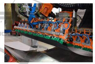
Figure 2: Both robots gripping a cutpiece.
