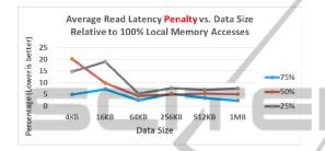
Figure 5: Average read latency penalty vs. data size with respect to 100% local access when the local portion of data varies from 75% to 25%
