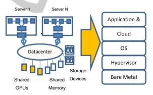
Figure 3: Software stack for accessing disaggregated resources.
