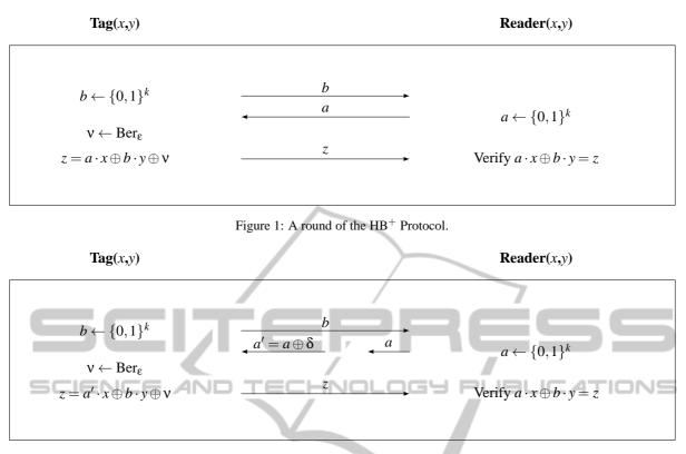
Figure 2: The GRS attack. The adversary adds a perturbation on the challenge vector *a* and looks if the whole authentication process will be disturbed or not.
