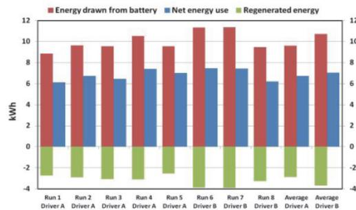
Figure 2: In-service electric energy consumption of a test bus running on Line 11, in city of Espoo.
