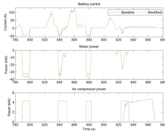
Figure 7: Simulated battery current, motor power and air compressor power for baseline and optimal air compressor operation during part of the cycle length.
