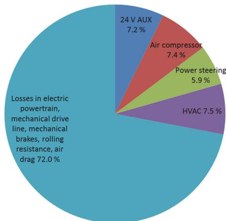
Figure 4: Measured share of auxiliary component energy consumption in electric city bus during real-life operation on Line 11 in Espoo, Finland at 15 °C ambient temperature.
