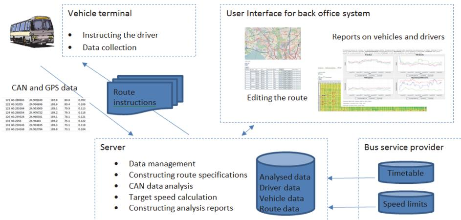
Figure 3: Communication between the components of the driver assistance system.
