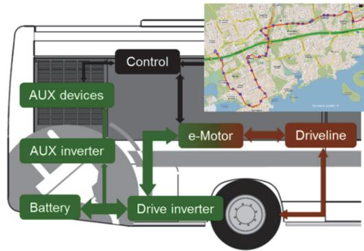
Figure 5: Subsystems of the auxiliary device energy consumption model. The coordinate data is included in the model, shown in a map at the top of the figure.
