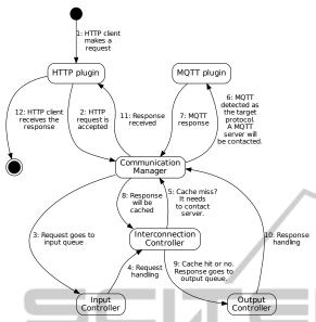
Figure 5: Collaboration diagram for a HTTP-MQTT request.
