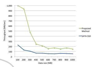
Figure 4: Comparison of read performance by Hadoop TestDFSIO with SCR enabled.
