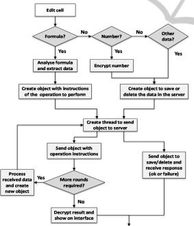
Figure 2: Client module flowchart according to user interaction.
