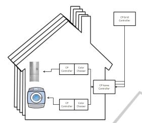
Figure 1: The architecture of the home system working with Deli2p and its interaction with the grid controller.
