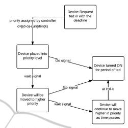
Figure 5: Flow chart describing the algorithm opertion on a single device.
