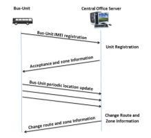
Figure 4: Sequence diagram of bus unit and server.
