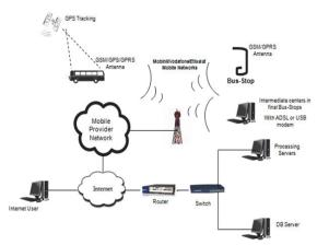
Figure 1: Main structure of proposed system.
