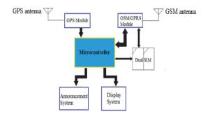
Figure 6: Block Diagram of in-bus unit.
