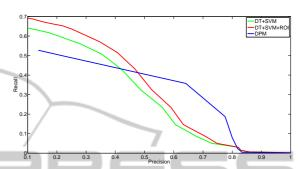
Figure 7: Recall-precision-curves for our detectors with (red) and without ROI extraction (green) and the DPM detector (blue).
