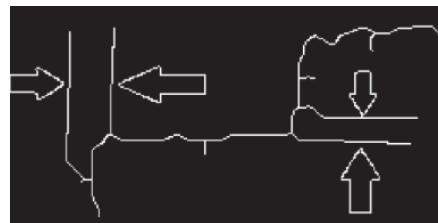
Figure 4: A portion of the edge thinned using fast parallel algorithm for thinning developed by Zhang and Suen, in 1984.
