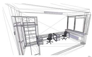
Figure 7: Wireframe view of the Room 215 model. Areas of high curvature have more triangles and appear as solid colours.
