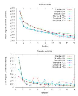
Figure 6: Mean angular deviation plotted against number of iterations for the Blade and Statuette.
