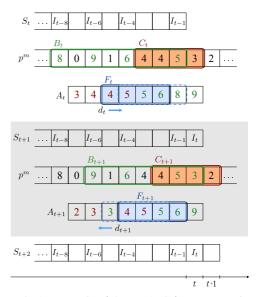
Figure 2: An example of the DWAFS frame processing for two successive frames  $I_t$ ,  $I_{t+1}$  with a windows of size w = 4. The sample windows  $C_t$ ,  $B_t$  and  $F_t$  (see text) are shown in red, green and blue respectively, the window shift of  $F_t$  is represented by the dashed blue window. In the case shown, frame  $I_t$  is selected while frame  $I_{t+1}$  is dropped (best viewed in color).
