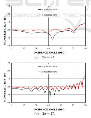
Figure 3: Monostatic RCS versus incidence angle for  $b = 0.05\lambda$ ,  $\varepsilon_r = 2.5 + i1.25$ ,  $\mu_r = 1.6 + i0.8$ .
