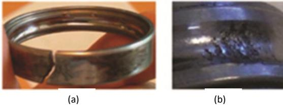
Figure 4: Bearing with fracture (a) outer ring failure and (b) inner ring failure (Source: (Medjaher et al., 2012)).
