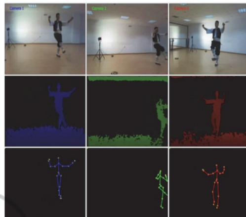
Figure 6: Traditional dance capture using multiple synchronized Kinect sensors.
