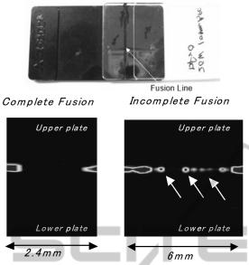
OCT target (Laser-fused plastic plate)
