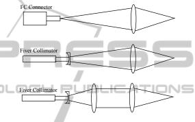
Figure 5: Optical probe assembly.
