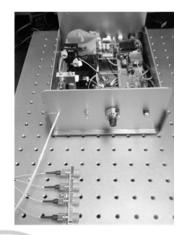
Figure 9: Multi-channel probes on a portable OCT.
