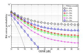
Figure 5: BEP as a function of the OSNR for 10 Gbit/s OOK crosstalk signal with M=4 and different duty-cycles.
