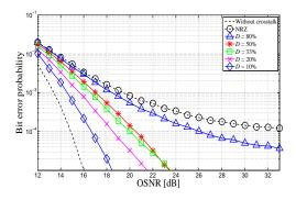
Figure 6: BEP as a function of the OSNR for 10 Gbit/s DPSK crosstalk signal with M = 4 and different duty-cycles.
