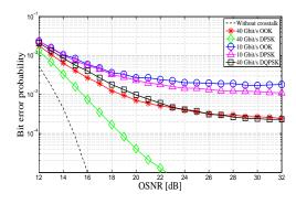
Figure 4: BEP as a function of the OSNR for M=8 interferers and different modulation formats and bit rates on the crosstalk signal.
