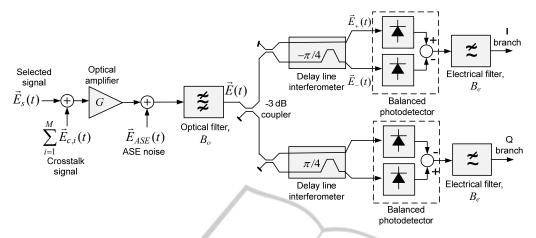
Figure 1: Block diagram of the DQPSK optical receiver.
