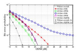
Figure 2: BEP as a function of the OSNR for a single interferer, M = 1 and different modulation formats and bit rates on the crosstalk signal.
