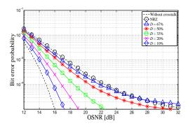
Figure 7: BEP as a function of the OSNR for 40 Gbit/s DQPSK crosstalk signal with M=4 and different duty-cycles.
