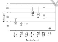
Figure 4: Box-and-whisker plot of latencies for the game *Shadowgrounds* per test case (sample size n = 250). The box indicates the 25th and 75th percentiles, whereas the whiskers mark the 2.5th and 97.5th percentiles. The median, i. e., 50th percentile, is denoted by a horizontal bar within the box.
