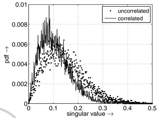
Figure 9: PDF (probability density function) of the ratio  $\vartheta$  between the smallest and the largest singular value for correlated (solid line) as well as uncorrelated (dotted line) frequency non-selective ( $4 \times 4$ ) MIMO channels ( $d_\lambda = 1/32$ ,  $\phi = 30^\circ$  rad and  $\sigma_\xi = 1,0$ ).
