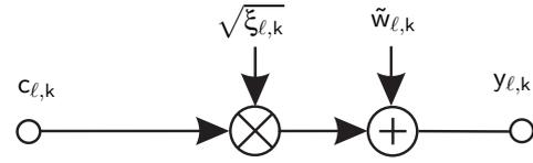
Figure 6: Resulting system model per MIMO layer  $\ell$  and transmitted data block  $k$ .
