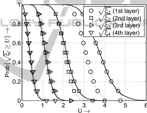
Figure 10: CCDF of the layer-specific distribution for correlated (solid line) as well as uncorrelated (dotted line) frequency non-selective ( $4 \times 4$ ) MIMO channels ( $d_\lambda = 1/32$ ,  $\phi = 30^\circ$  rad and  $\sigma_\xi = 1,0$ ).
