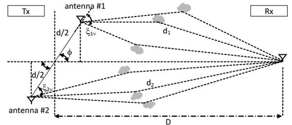
Figure 2: Antennas' physical disposition: two transmit and one receive antennas in a scattered environment.
