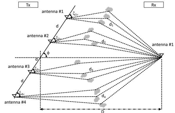
Figure 7: Antennas' physical disposition:  $(4 \times 4)$  MIMO with neighbour transmit antennas correlation.
