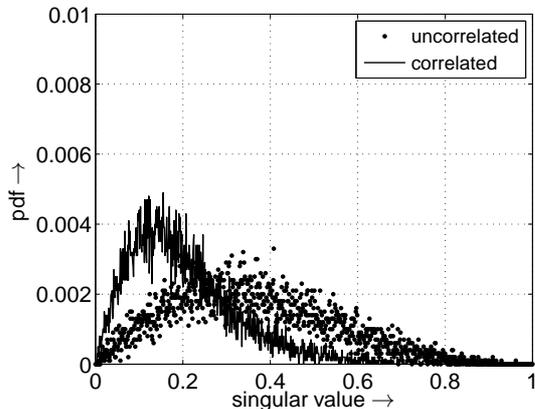
Figure 8: PDF (probability density function) of the ratio  $\vartheta$  between the smallest and the largest singular value for correlated (solid line) as well as uncorrelated (dotted line) frequency non-selective ( $2 \times 2$ ) MIMO channels ( $d_\lambda = 1/32$ ,  $\phi = 30^\circ$  rad and  $\sigma_\xi = 1,0$ ).
