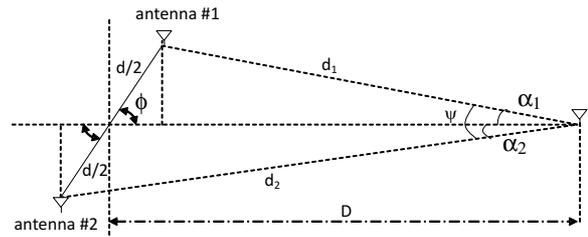
Figure 1: Antennas' physical disposition: two transmit and one receive antennas.
