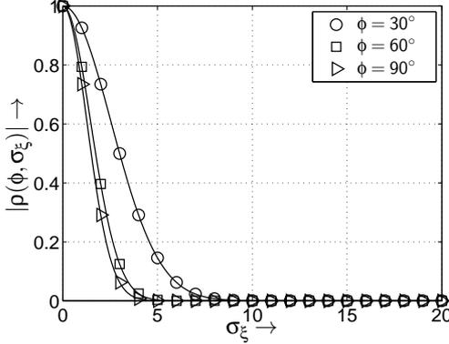
Figure 5: Dependency of  $|\rho(\phi, \sigma_\xi)|$  as a function of  $\sigma_\xi$  and  $\phi$  assuming a wavelength specific antenna separation of  $d_\lambda = 1/8$ .
