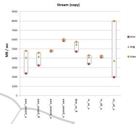
Figure 1: STREAM (copy) benchmark across four infrastructures. Labels indicate provider (e.g. aws for Amazon), region (e.g. useast is Amazon's US East) and distribution (u for Ubuntu, R for RHEL).
