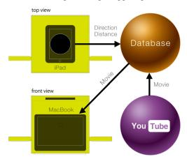
Figure 4: The system configuration diagram.
