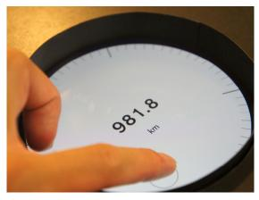
Figure 2: The dial for setting distance.
