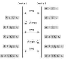
Figure 7: Synchronization test with two devices and no conflicts. Time flows from top to bottom.
