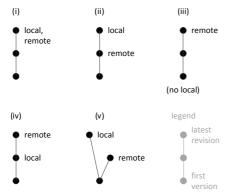
Figure 4: Revisions: do nothing (i and ii), get remote application information (iii and iv) and conflict resolution needed (v). Time flows from bottom to top.
