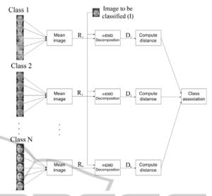
Figure 2: Scheme of the proposed image processing procedure.
