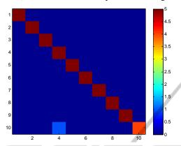
Figure 7: Confusion matrix for the Frobenius norm distance measure, image size of 17 x 20 pixels and only the first 10 subjects of the database. Dark colour indicates good classification (5 over 5 images well classified) for the given class. Only one image was misclassified.
