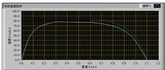
Figure 5: Braking curve of the train.
