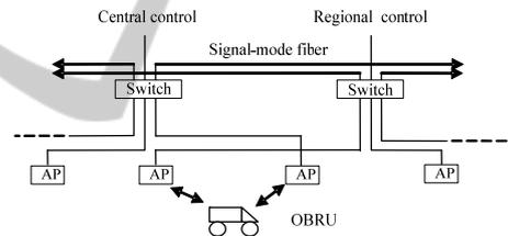
Figure 3: Schematic diagram of wireless data communication network.
