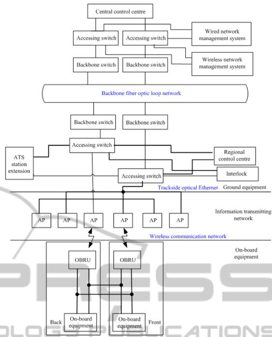
Figure 2: General model of ATP system.
