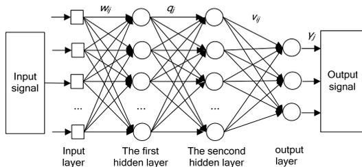
Figure 3: Structure of BP NN with several layers.
