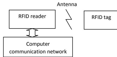
Figure 2: RFID Reader Block Diagram.
