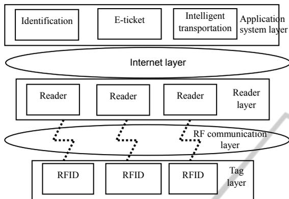
Figure 3: System of RFID-based Internet of Things.
