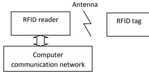
Figure 2: RFID Reader Block Diagram.
