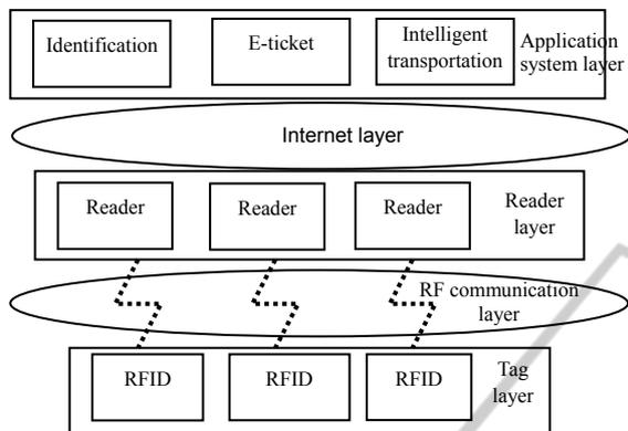
Figure 3: System of RFID-based Internet of Things.
