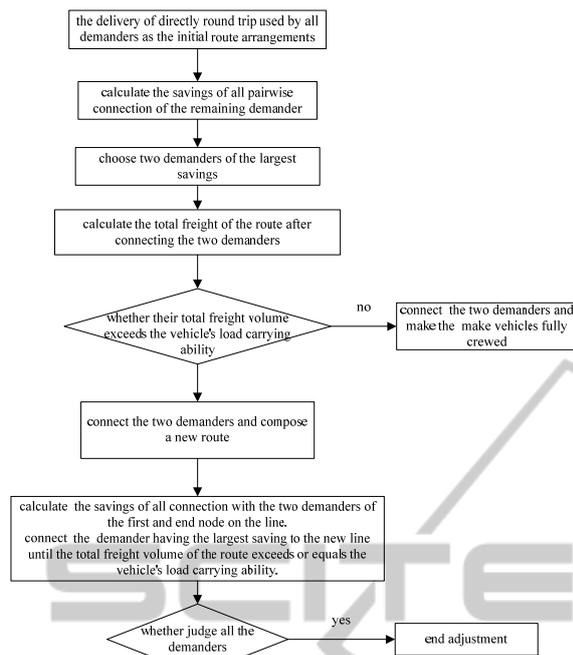
Figure 4: The flowchart of optimization algorithm (Xuezhi and Gongyu, 2008).
