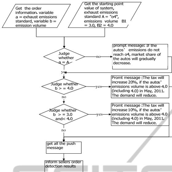
Figure 5: flowchart of ecological detection algorithms
