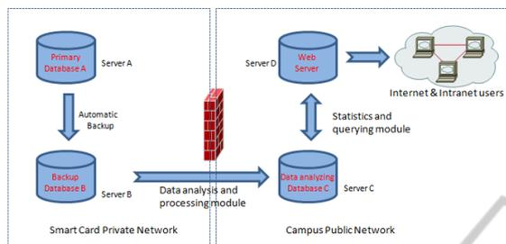
Figure 1: Architecture of the data analysis system.
