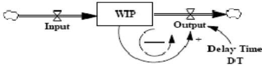
Figure 1: Structure of linear first-order system with negative feedback.
