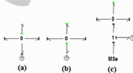
Figure 1: (a) Sensor e in behavioral model, (b) inverted causality in e and (c) substituted representation for inverted causality in e.
