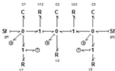
Figure 7: BG model in preferred differential causality.
