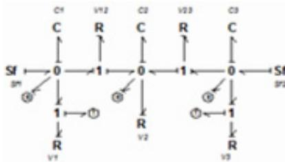
Figure 6: BG model in preferred integral causality.
