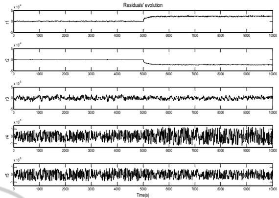
Figure 11: Residuals evolution in case of V12 fault.
