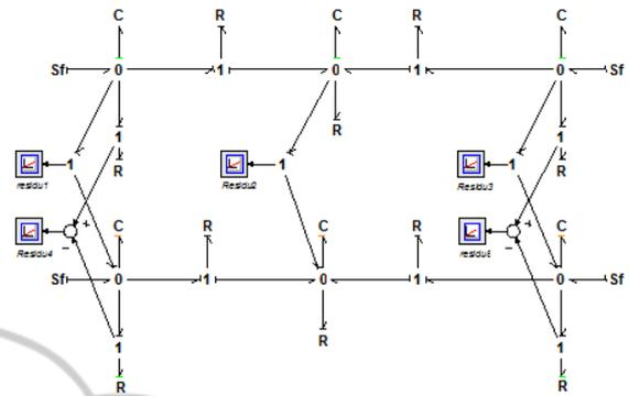
Figure 8: DBG of the three tanks system.
