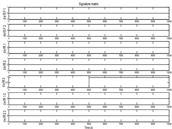
Figure 15: Fault indexes with fault signature matrix.
