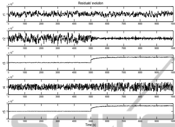
Figure 14: Residuals evolution in case of V3 fault.
