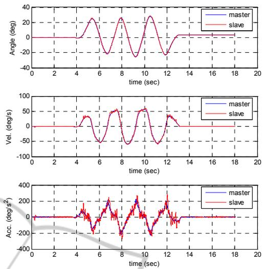
Figure 9: Position tracking results during axis 1 motion where the slave arm with a payload of 10 kgf follows arbitrary motion of the master.
