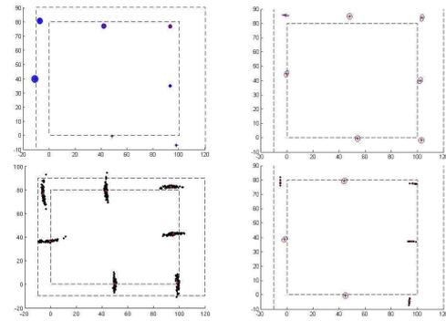
Figure 5: Predicted positions of the robot (top left), positions estimated from visual landmarks (top right), positions estimated from RFID tags (bottom left), positions estimated from the fusion (bottom right).
