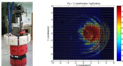
Figure 1: The RACKHAM demonstrator from LAAS(left), Cartesian Detection Model of every RFID antenna (right).
