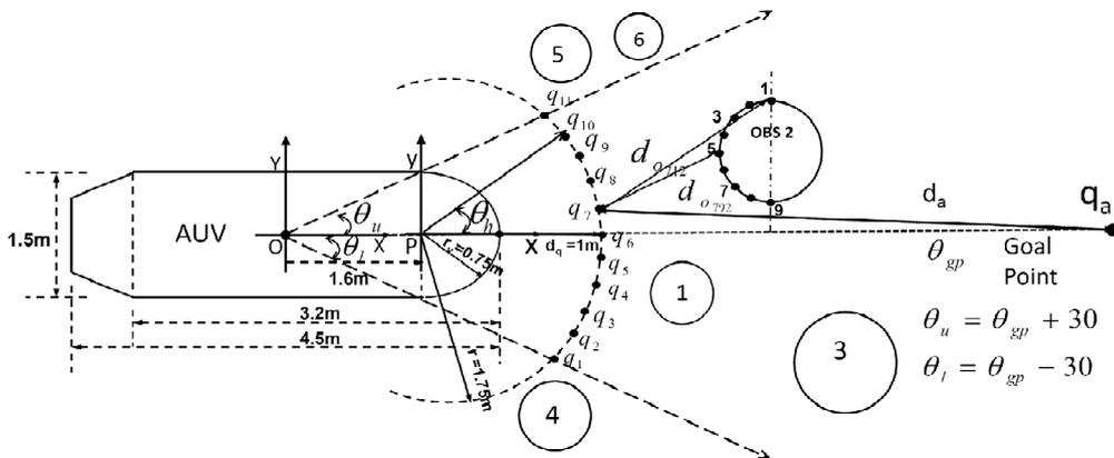
Figure 5: Methodology for the implementation of 2D obstacle avoidance algorithm.
