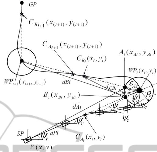
Figure 1: Calculation of heading correction for smooth turn during course change at waypoints.
