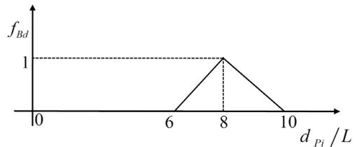
Figure 3: Distance factor for the auxiliary point  $B_i$ .
