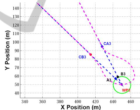
Figure 8: Close-up view of the modified waypoint guidance by LOS at waypoint 3.
