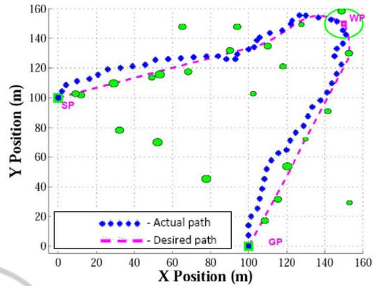
Figure 12: Obstacle avoidance for the obstacles of various sizes in the desired path with the improved waypoint guidance data.
