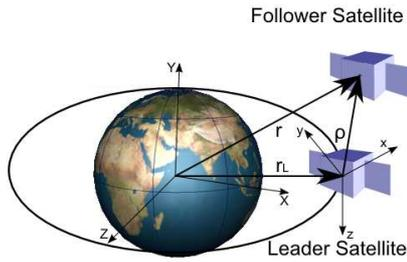
Figure 1: Geometry of orbit motion of leader and follower satellites.
