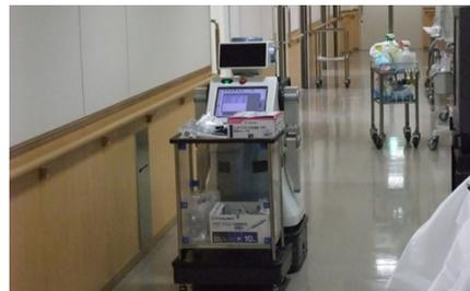
Figure 1: An autonomous robot for hospital use.
