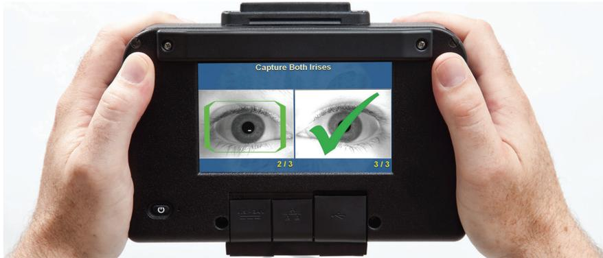
Figure 1: The military mobile iris based identification system HIIDE 5.
