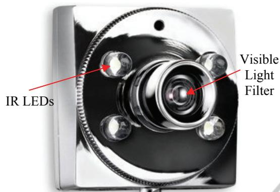
Figure 4: The modified camera.
