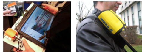
(a) Tablet PC with Camera and inertial sensor (b) GPS receiver
