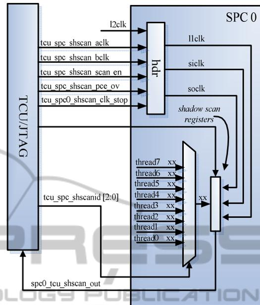
Figure1: The Shadow Scan Architecture.
