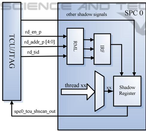
Figure 3: The Datapath of Improved Shadow Logic with IRF.
